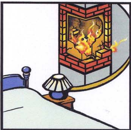
Increased Risk from a Chimney Fire
